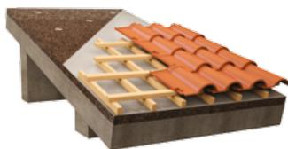
PITCHED ROOF WITH ROOF MEMBRANE SYSTEM
