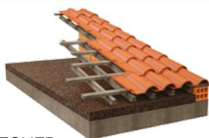
PITCHED ROOF WITH RIGID INSULATION OVER SLAB
